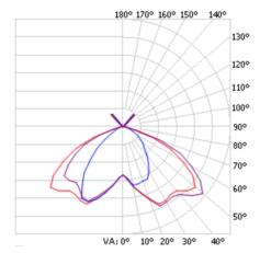
**LED Lamp** Luminous Flux 8851 lm 2700 K Colour temperature CRI 80 3 Step MacAdam Ellipse Nominal Power 80W **Beam Angle** Asymmetrical
